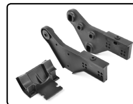
C-00180-296 Wheelie Bar Mount - Left-Right - Composite - 1 set
