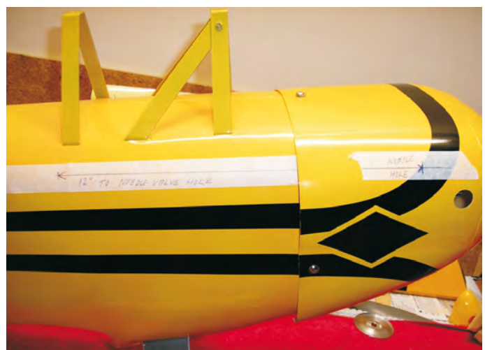
Masking tape makes it easy to check measurements to fit the cowl and place the needle valve opening in the correct spot.
