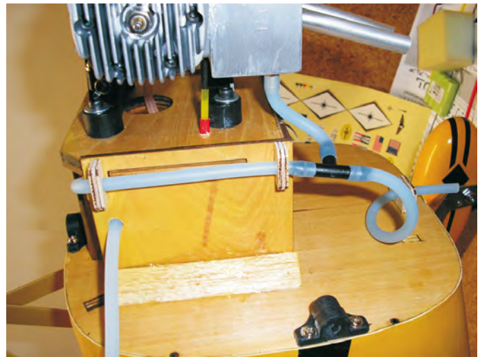
A little bit of Marriner engineering expertise is applied to the plumbing. A fuel bung is inserted into the vent at the bottom and removed for filling.
