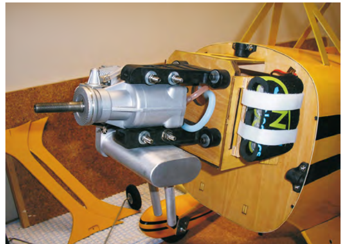
With the battery pack mounted up front the the centre of gravity was spot on.
