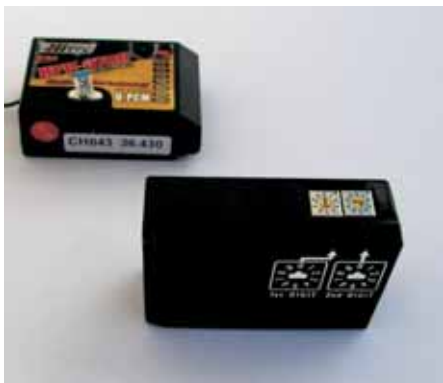
Change the channel with two rotary dials on the optional synthesised transmitter module. Behind is the new dual conversion PCM receiver.
