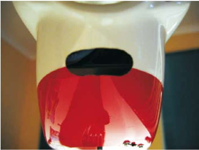
Extra vent added to cowl to flow air over ESC.
