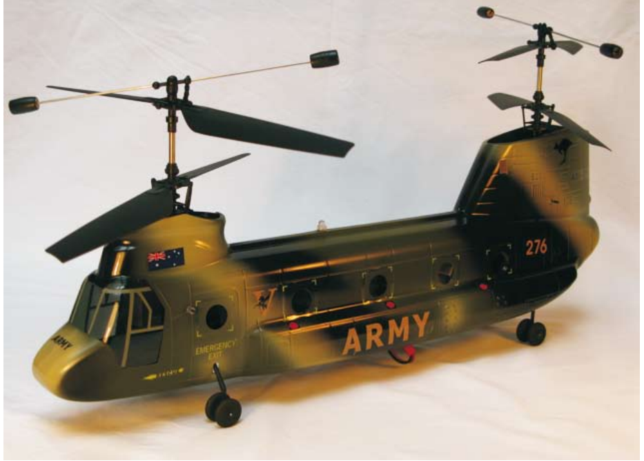
Rotor diameter 340 mm, weight 400gm, 3s LiPo, 4 channel ready to fly.
