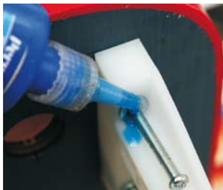
Loctite holds bolts where they should.
