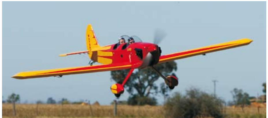
Wingspan: 2100mm, Length: 1490mm, Weight: 5kg, Engine: 120 - 150 4 stroke.
