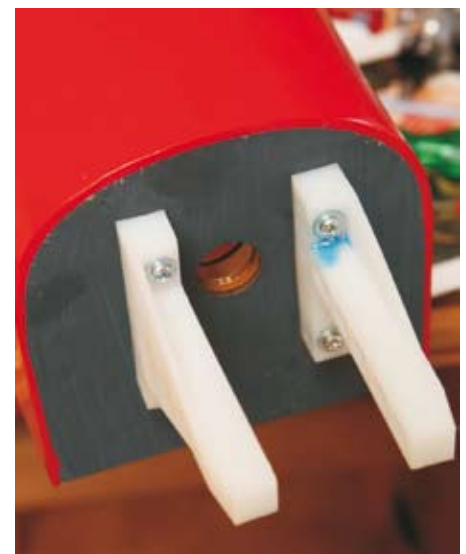
The Space Walker will take a wide variety of engine sizes. Space the two piece nylon engine mount for your engine then drill the fire-wall.
