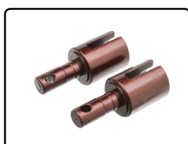
C-00180-154-X PRO Centre Diff. Outdrive Cup - Swiss Spring Steel - 2 pcs
