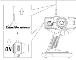
Make sure no one is using the same frequency. Turn on transmitter first, then turn on the receiver. Check the throttle and steering functions and check the radio range before starting the engine. If you switch on the R/C car first before the transmitter, you may lose control of the R/C car.
